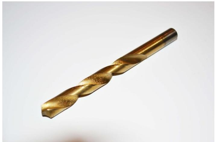
**Photo 1: ½” twist drill bit; the largest size that model railroaders will commonly use.**
