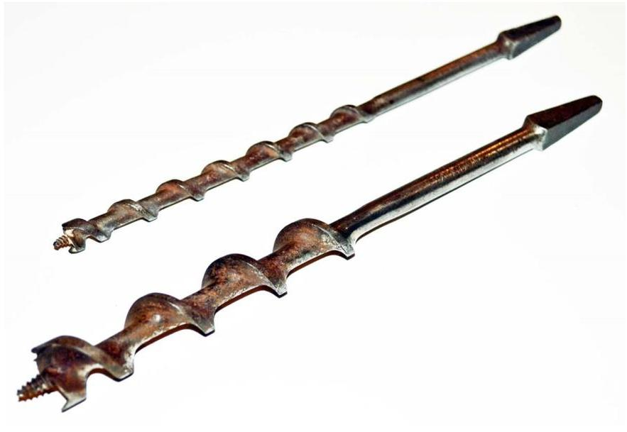
**Photo 4: Auger bits with a four-sided tapered shaft end for use with a hand brace.**
