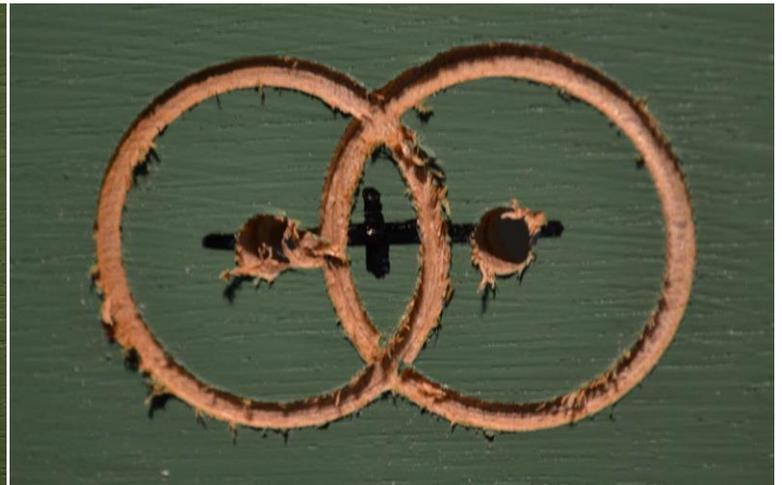
*Photo 5: Both holes are partially drilled, switching back and forth between them*
