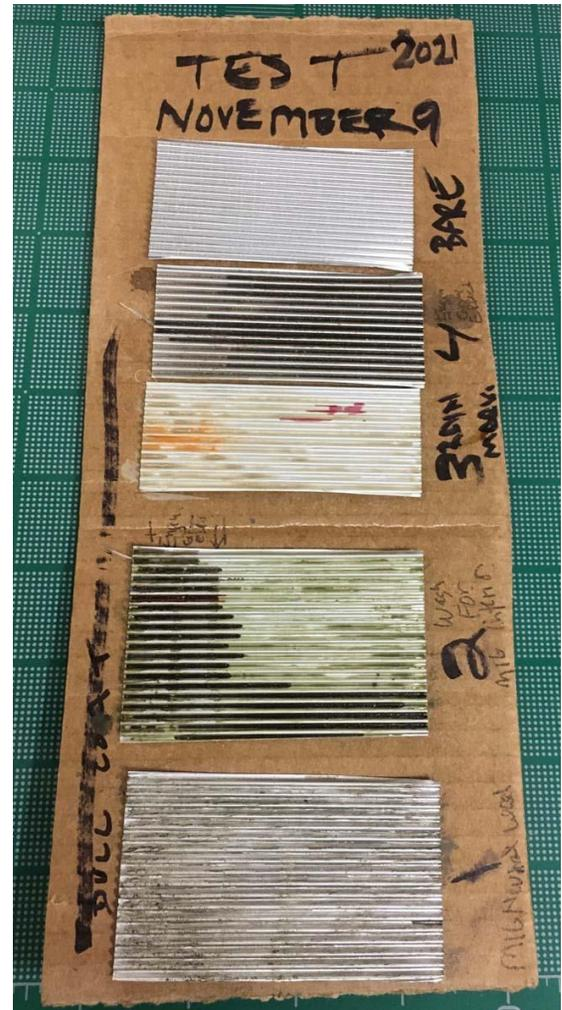
**Photo 4:** The cardboard that was used to identify which paint was used where. While one might suppose that one would easily recall which paint was used on which sample panel, that is not the case. I used hot glue to affix the panels to the cardboard. I marked each cardboard holder with a black magic marker being careful to use the paint number and name for clarity (good where the paint names are similar to prevent any confusion)
