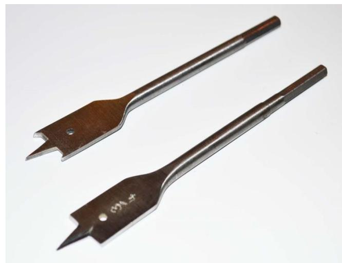
**Photo 2: Flat spade drill bit lower and a spade drill bit with extra points top.**
