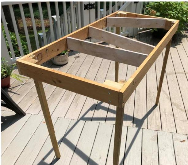
**Photo 1. Module frame, legs temporarily attached**
