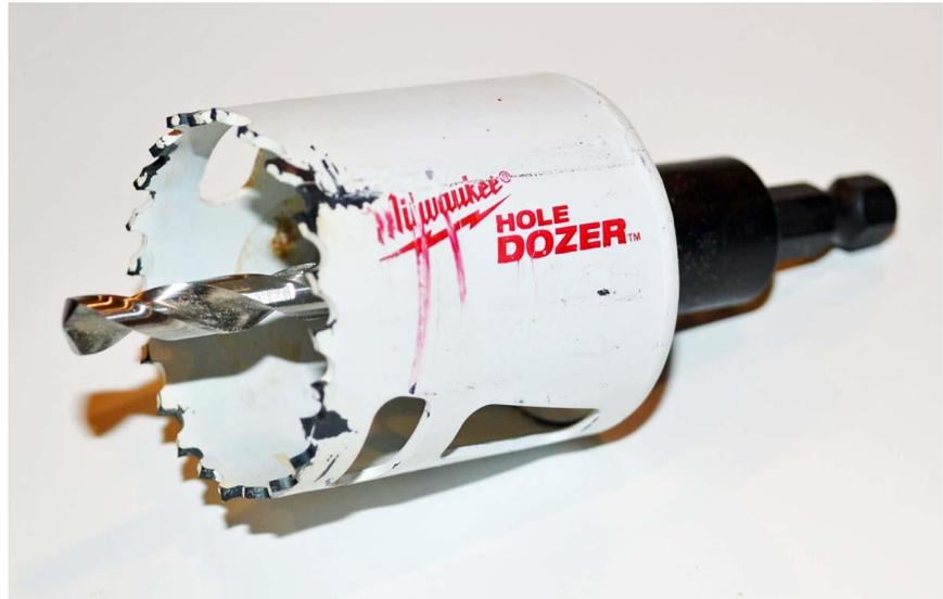
**Photo 5: Hole saw blade and arbor with pilot drill.**
