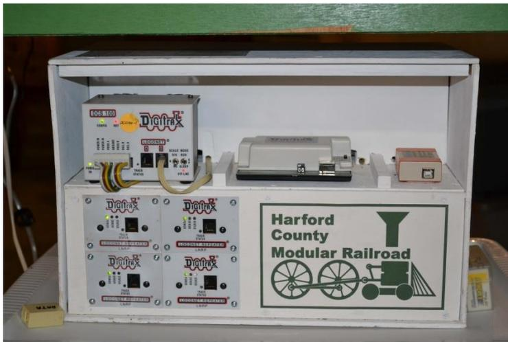
*Photo 10: The LNRP panel installed as part of a DCC control system for a large modular railroad.*
