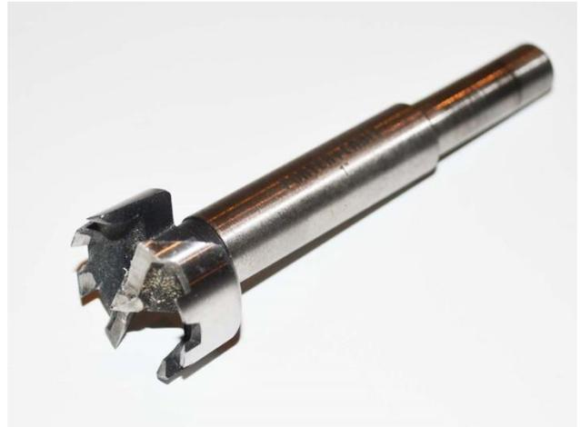
**Photo 3: Forstner drill bit. Notice the many cutting surfaces in the middle, the periphery, and in between.**
