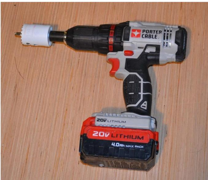
The only tools that you need are a drill motor, a 1 ½” hole saw, and a ruler (**Photo 1**). Additionally, a small level will aid horizontal alignment. If you don't have a 1 ½” hole saw, it can be purchased for about \$10 at a local hardware store. A hole saw is much more controllable for drilling the overlapping holes than other types of bits and is less likely to damage the wooden fascia by splintering.
