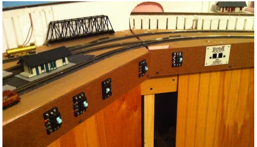
Photo 7: Fascia made with hardboard. Turnout switches and Digitrax Loco-Net plug-in IR receiver have been installed.
