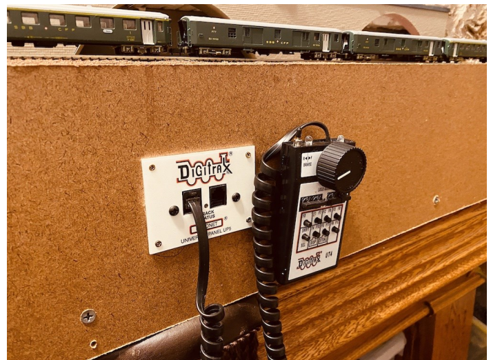
Photo 9: Digitrax IR receiver plug-in and walkaround throttle mounted on the side of the peninsula.
