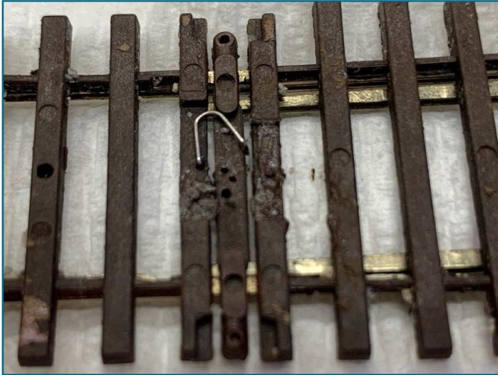
*Photo 2 – The tiny U-shaped spring is normally covered by a small plastic square, which holds it in place. During the move, the plastic came off, which must have allowed the spring to come loose of the throwbar. This happened on the first two turnouts of the yard ladder.*
