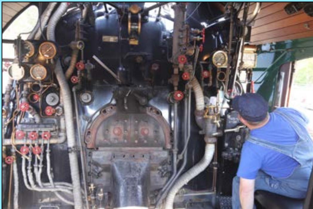
*Photo 12: Priming the injector under the cab; the fireman is reaching down to the valves on the floor.*
