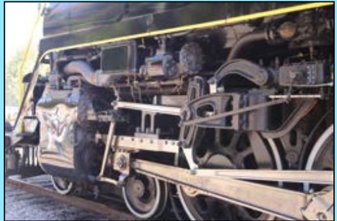
*Photo 17: Valve Gear, Worthington SA pump*
