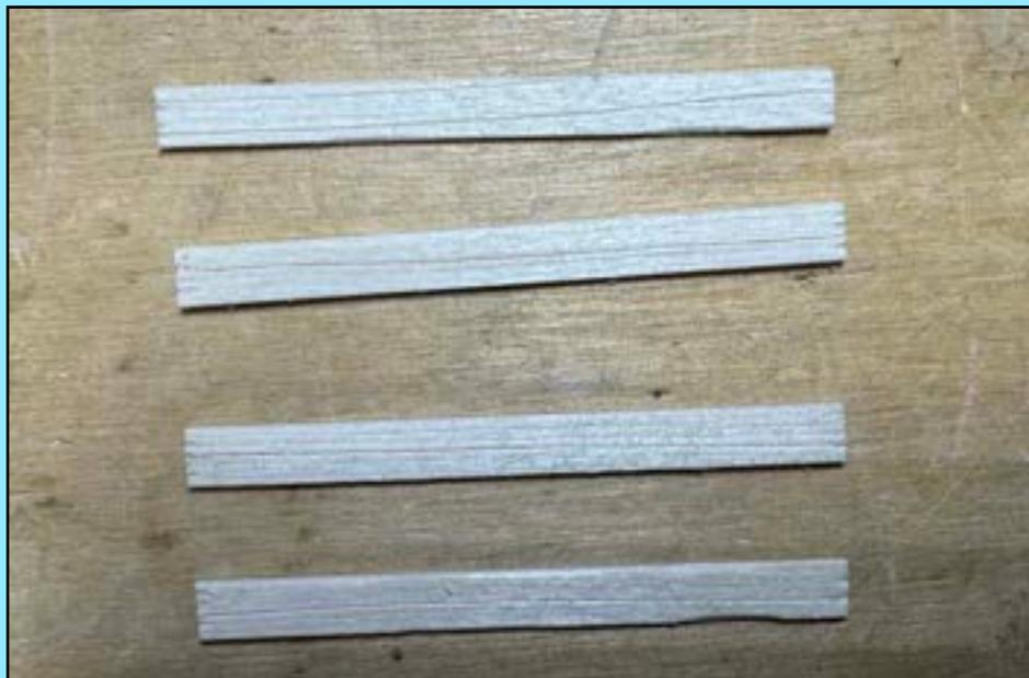
*Photo 6: Carved edge chamfers and roughed up board ends.*
