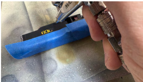
Photo 4 and Photo 5: The air eraser is shown here working its magic to remove the factory lettering and finish. It is sometimes necessary to work very close to the model for precise control. Eye protection and a face mask are highly recommended, as the abrasive compound tends to spread everywhere during the process.
