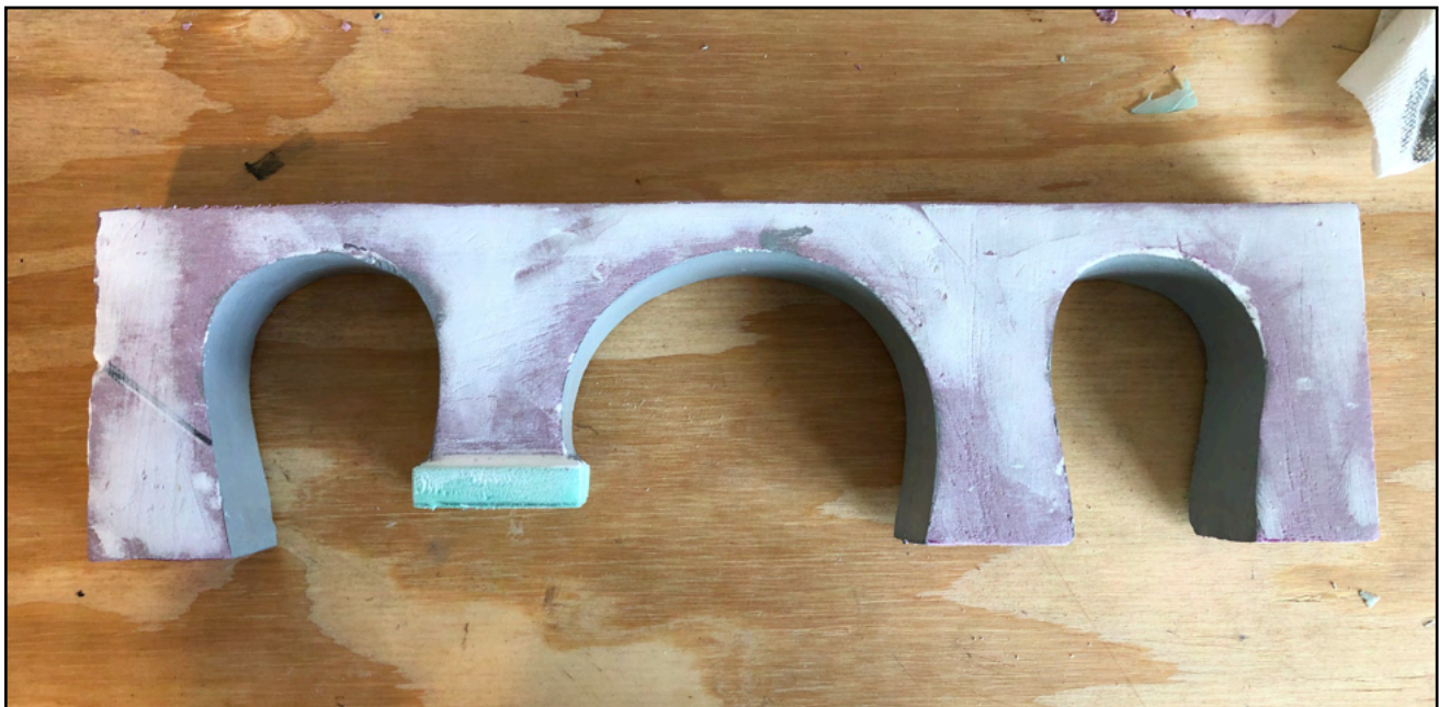
Photo 3: Basic Viaduct Shape Carved from 2-inch Thick Foam
