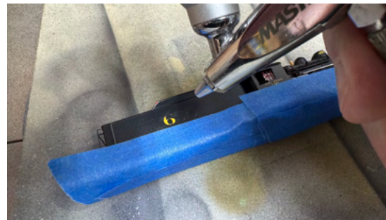
Photo 4 and Photo 5: The air eraser is shown here working its magic to remove the factory lettering and finish. It is sometimes necessary to work very close to the model for precise control. Eye protection and a face mask are highly recommended, as the abrasive compound tends to spread everywhere during the process.
